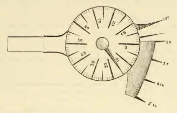
Mr. Eckley Coxe has had a useful addition made to his instruments in the shape of a set of removable rings, divided for 100ths, 1000ths, 66ths, 33rds, &c., &c. Two little serews hold the ring in place, whichever one may be in request for any particular plotting. When plotting on the scale of some other unit of distance is required another ring is substituted.
